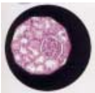
Image of field diaphragm is focused but not centered
