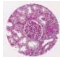
In this example the aperture is stopped down too far, and the image has very high contrast and appears "grainy". There is an inverse relationship between contrast and resolution.
