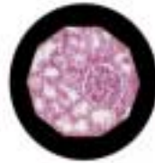
Image of field diaphragm is focused and centered
