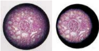
Image of the field diaphragm is out of focus and not centered
